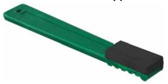
TETRABOR hand lappers are sintered from pure boron carbide without binding agents. Boron carbide is the hardest material after diamond, which is why Tetrabor hand lappers have extremely high abrasion resistance, and minimal wear. They are very economical in use. Fixed with synthetic resin on a plastic handle, Tetrabor hand lappers are ideally suited for dressing and resharpening hard metal as well as high speed tools.
