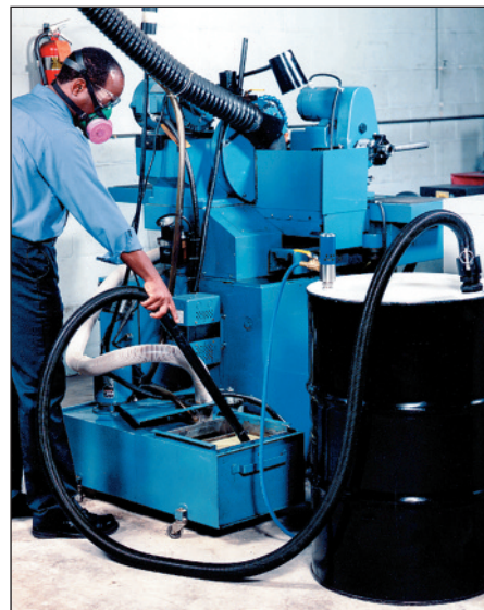
The Royal PneuVac pump filled this 55-gallon drum with coolant in less than two minutes.
