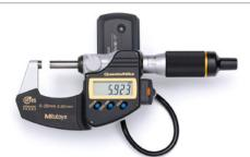
Electronic data collection allows the user of the gage to send the measurement displayed on the gage directly to a computer by simply pushing a data send button. An incredible variety of Data Management is available. From USB cables and multiplexer systems to wireless systems, MeasurLink® can support them all.
