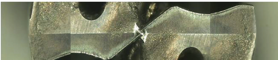
Competitor A (After Drilling 546 Holes)
