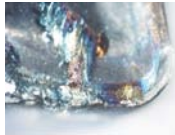
Built-up edge (Adhesive wear)
