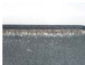
Thermal cracks (Thermal wear)
